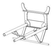
STEP 5 – Bolt the winch handle to the winch and assemble the wheels, wheel washers and cotter pins.
