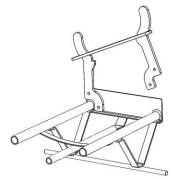
STEP 4 – Bolt the second cradle arm to the frame and tighten all the bolts.
