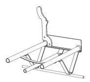
STEP 2 – Insert the other cradle arm through the one slot in the cross bar. The cross bar will rest on the small landing of the cradle arm.
